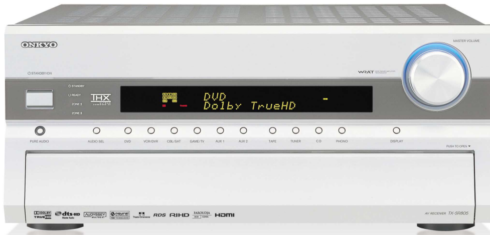
The lesser-used controls are neatly tucked away behind the drop-down panel.
