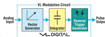
The upper and lower portions of the spike noise waveform are symmetrical, so they have the same area. Therefore, if the analog signal contains spike noise, their charge quantities will cancel each other out. This will ensure accurate pulse width modulation at all times. Onkyo's third-generation VL Digital technology includes an inverted Darlington circuit that goes beyond earlier versions to accurately produce a current flow based on the input voltage.
