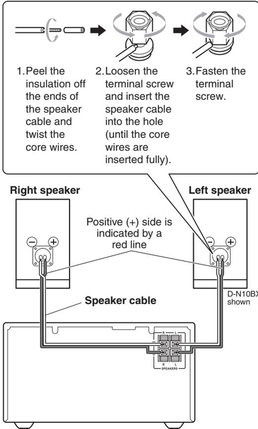
The type of speaker terminals used on the receiver and their position depends on the model. Refer to the receiver's instruction manual for details on connecting speakers to the receiver.
