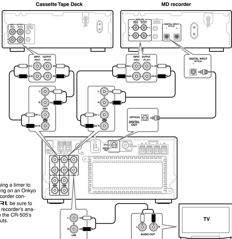
**Note:** If you are using a timer to start recording on an Onkyo Mini Disc recorder connected via **RI**, be sure to connect the recorder's analog inputs to the CR-505's analog outputs.
