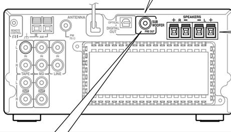
The SUBWOOFER PRE OUT should be connected to the input on your powered subwoofer. If your subwoofer doesn't have an amp built-in, you'll need to use an external amp. See the manual supplied with your subwoofer for more information.
