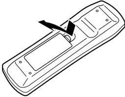
**2** Insert the two supplied batteries (AAA/R03) in accordance with the polarity diagram inside the battery compartment.
