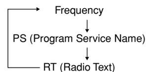
When the CR-505 receives RT information, “WAIT” appears on the display first, and then the received text scrolls across the display.
