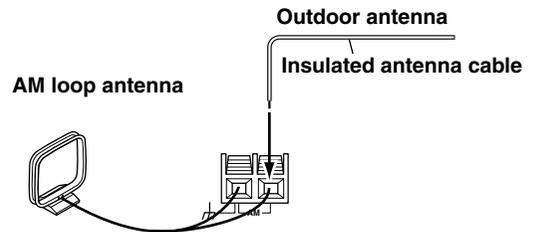
Outdoor AM antennas work best when installed horizontally outside, but good results can sometimes be obtained indoors by mounting it horizontally above a window. Note that the AM loop antenna should be left connected. Outdoor antennas must be grounded in accordance with local regulations to prevent electrical shock hazards.
