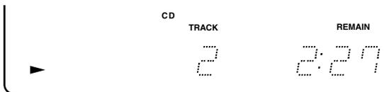
**Remaining disc time:** The amount of time remaining for the entire disc (REMAIN and TOTAL indicators appear).
